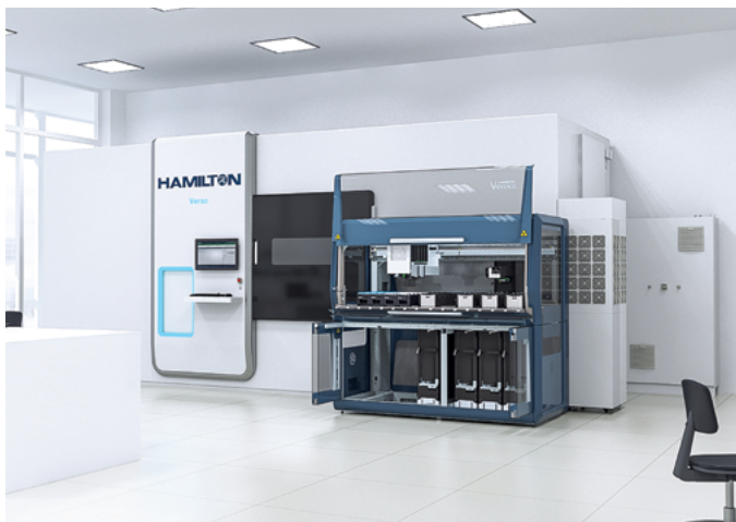
Verso integrated with Microlab VANTAGE Liquid Handling System.
