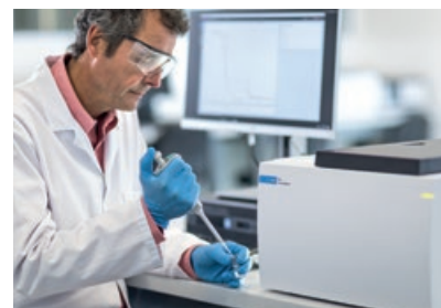
Cary 3500 double beam, multicell, UV-Vis spectrophotometer
